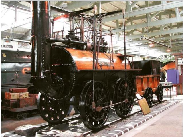
metals and plans and anecdotes. The boiler on the original had only one fire tube which was inefficient and eventually spelt doom to the original; Jonathan fitted about thirteen tubes. The inefficient first full sized boiler exploded unfortunately
